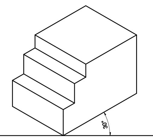
Candidates must use the correct Set Square. Sale can be estimated but the steps should be higher than deeper. The top step is not as high as the other two.
