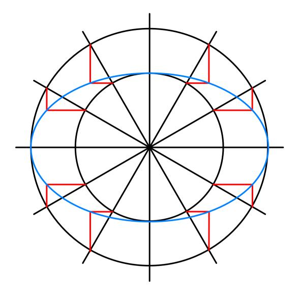
Candidates should complete all the construction lines correctly. Maximum of 3 marks for correct construction lines. The Ellipse should touch all of the relevant points to gain marks up to a maximum of 3.
